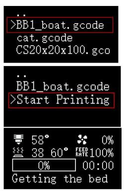
The nozzle and the heated bed start to warm up, and when the temperature reaches the preset temperature, the machine starts printing.
